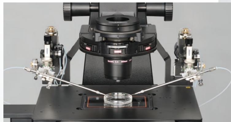
With pipette angle set to 20 degrees (low)
